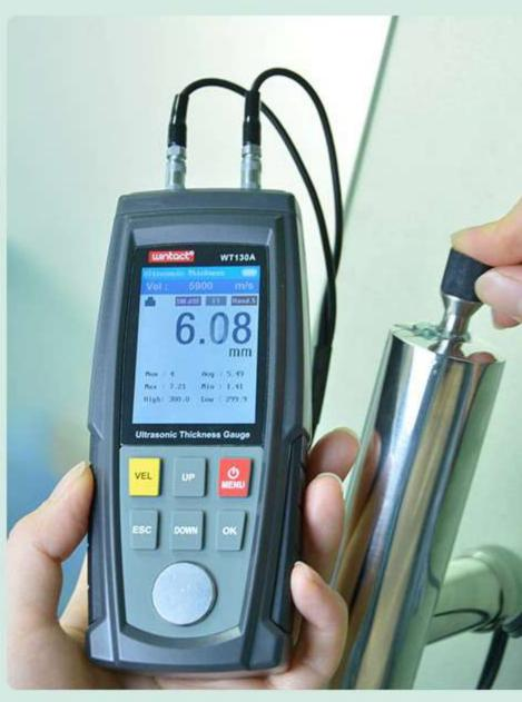
It is transmitted at a constant speed and can distinguish waves reflected from the back side for this instrument.
