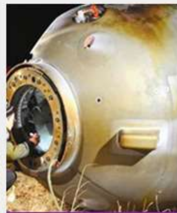
Thermal insulation coating
